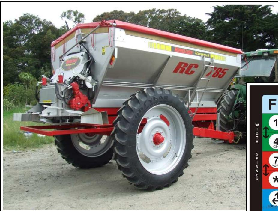
High clearance, twin chain drive system for ultimate control of spreader. Computer option available
