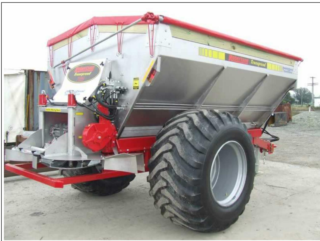
For large volumes of waste, wet or dry lime and light rates of urea, the **Transpread 730 PROspread** will spread most materials. A 730 mm wide door opening gives unobstructed feed on to the high powered 675 mm spinners. High floatation tyres keep you on top in the wet and prevent you ploughing the corners of the fields.
