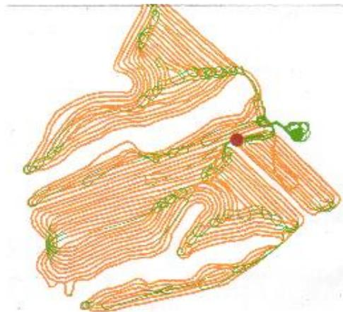
The GPS systems currently available through competitors are only able to map, or change the over all rate based on the GPS position. The pictures shown here were taken by GPS software showing that even with the best GPS guidance, a driver still has to drive to the conditions. These unavoidable errors cannot be adjusted for, except with a Transpread Twin Chain spreader. By adding GPS technology to older spreaders, they will not be able to take advantage of this innovative, patented technology.
